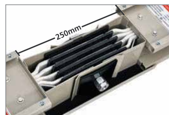
Step 3: Insert the Joint Block in between two adjacent Feeders and ensure equal contacts on both side of Joint Plates. After jointing ensure gap between enclosure of two elements is 250mm
