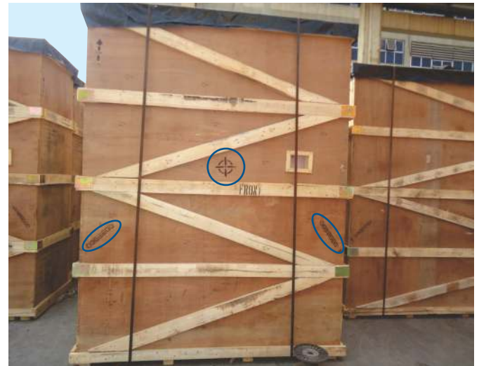
Figure 11 - Chain marks on packed TUs
